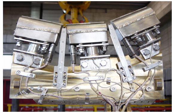
Fig. 1. Photograph of three units of lithium limiter installed on the support used for the LLL introduction inside FTU from the bottom vertical port. The dimensions of each unit of the LLL are: length = 100 mm, width = 34 mm. The two Langmuir probes are visible in the interspace between units.
